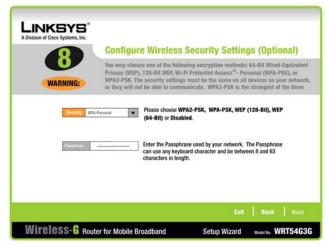
Figure 5-12: Configure Wireless Security Settings - WPA-PSK Screen
